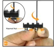
17.1. Hold the Keymod Nut in place and loosen the screw by turning it counter-clockwise with the included 3/32" Allen Wrench. Do not fully detach the Keymod Screw from the Keymod Nut.
