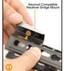
11.On the Keymod Compatible Receiver Bridge Mount, hold the Keymod Nut in place and loosen the screw by turning it counter-clockwise with the included 3/32" Allen Wrench. Do not fully detach the Keymod Nut.
