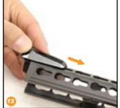
12. Place the Keymod Compatible Receiver Bridge Mount onto the last Keymod Slot of the lower handguard rail. Insert the nut through the larger portion of the Keymod slot. Ensure the protruding foot of the nut is pointing toward the muzzle of the firearm. Slide the Keymod Compatible Receiver Bridge Mount toward the muzzle until the mount fully drops into the handguard.
