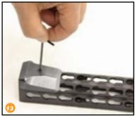
13. Once the Keymod Compatible Receiver Bridge Mount fully seats into and engages the handguard. Tighten the screws on top of the bridge mount to lock it securely on the handguard.
