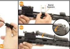
15. Loosen the Barrel Spacer screws. Place the Barrel Spacer onto the barrel at the position (A). Install the gas tube over the Barrel Spacer. Lock the gas tube down by pushing the gas tube lever downward. Tighten the 2 screws to lock the spacer firmly. The Barrel Spacer will prevent over tightening of the top/ bottom covers and allow for normal operation of the piston.
